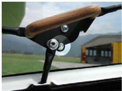
Correct - door secured
